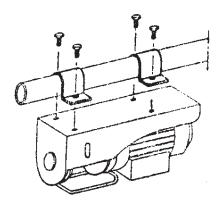
Figure 1. Mounting the Hoist.
